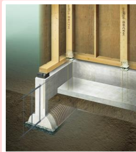
Direct foundation joints
