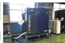
New compressor in the ironworking plant
